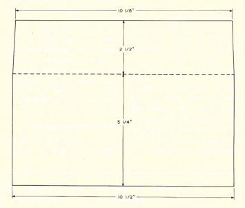
Fig. 4. Pattern for the rear cover of Comprint. Make the cover from heavy non-corrugated cardboard. Score with a sharp knife at the fold. After folding, put some vinyl shelf paper on the cardboard. Attach at the rear to the inside rear cover with adhesive tape. The cover prevents the paper from curling back into the printer mechanism.
